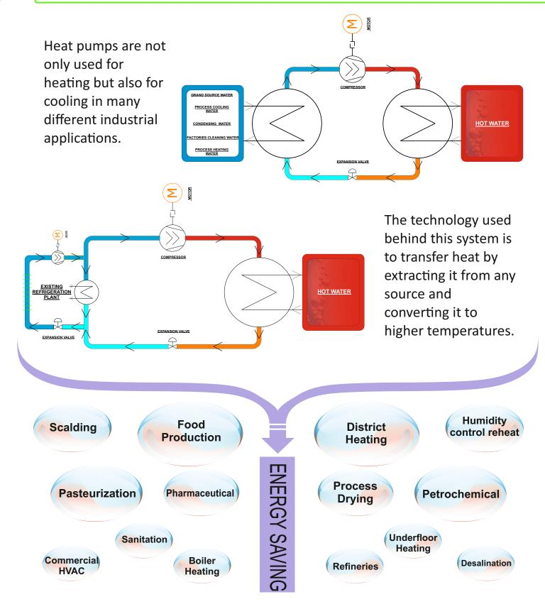
The technology of the heat pump is used in recovering waste heat and to raise its temperature to more useful levels allowing significant potential for energy saving.
